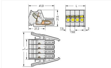
Dimensions in mm L = (pole no. - 1) x pin spacing + 10.5 mm L1 = L + 23.7 mm
