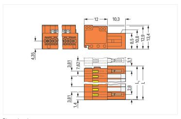
Dimensions in mm L = (pole no. - 1) x pin spacing + 5.9 mm + 0.45 mmL1 = L - 0.45 mm
