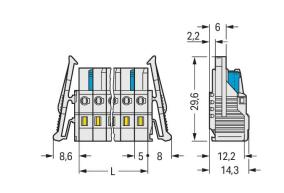
Dimensions in mm L = pole no. x pin spacing 2-pole female connectors – one latch only
