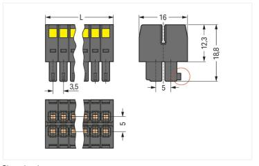
Dimensions in mm  $L = \hbox{(pole no./2)} - \hbox{1] x pin spacing + 5.2 mm} \\ \hbox{Coding finger (red circle)}$
