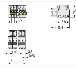
Dimensions in mm L = pole no. x pin spacing
