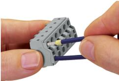
Solid conductors  $\geq 0.5 \text{ mm}^2$  (20 AWG), as well as ferruled, fine-stranded conductors can be terminated by simply pushing them into unit. Integrated test ports allow touch contact with current bar via test probes in both horizontal and vertical directions.
